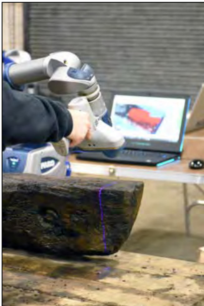
Laser scanning a ship timber. (Credit: Alexandria Archaeology)
